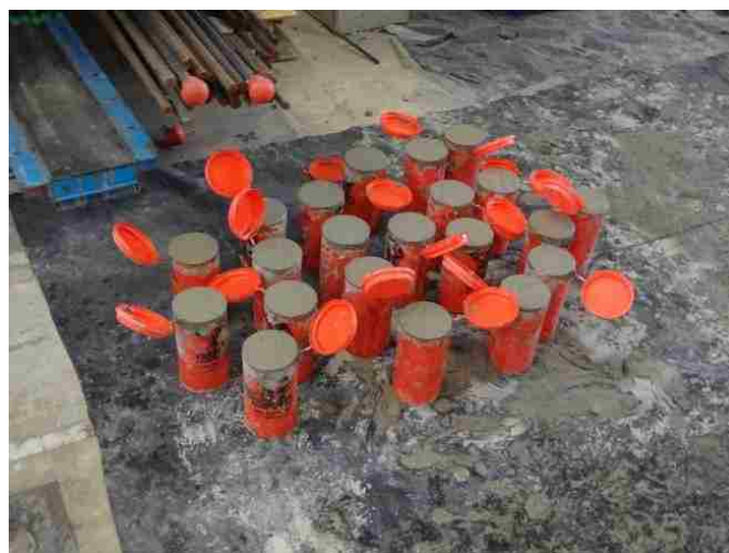
Figure 3.15. Test Girder CIP Deck QC/QA Specimens
