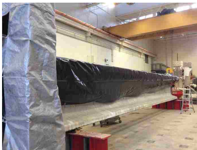
Figure 3.16. Tarping of CIP Deck
