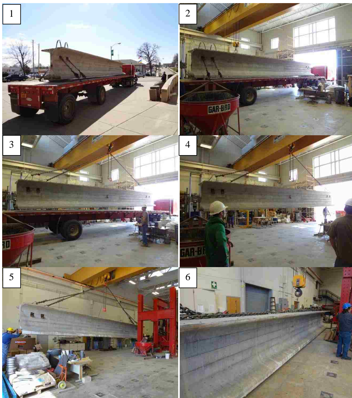
Figure 3.11. Test Girder Delivery Process at Missouri S&T
